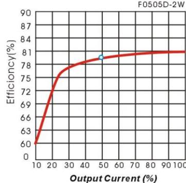
Efficiency VS Output Load curve
