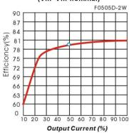
Efficiency VS Output Load curve (Vin=Vin-nominal)
