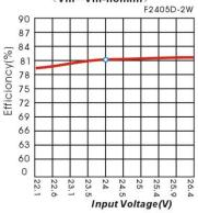
Output Load VS Efficiency curve (Vin=Vin-nominal)
